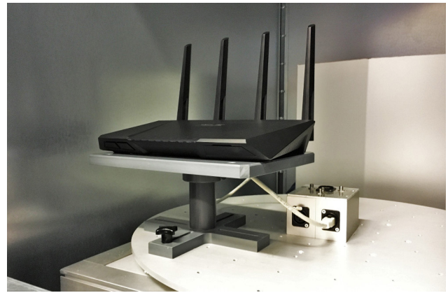
4. DUT access point with 4x4 MIMO
